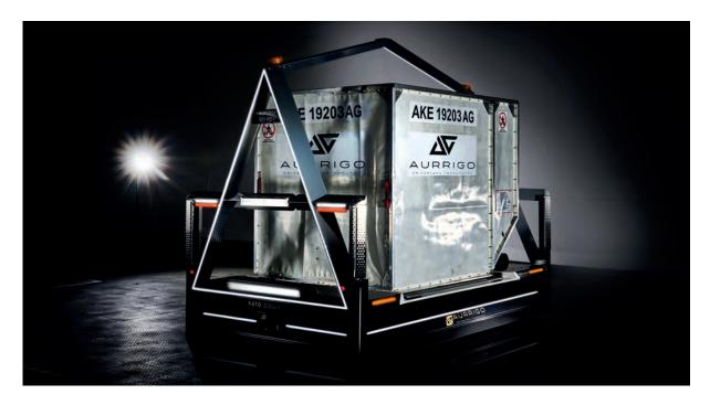
The rechargeable, battery powered Auto-Dolly, is designed to replace the fleets of diesel and electric tug vehicles, all of which are manned, and deployed in considerable numbers at commercial airports globally.
