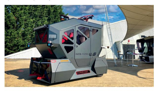
The Auto-Patrol core structure and platform is similar to that of an Auto-Pod, however it has been bolstered with security focussed technology, including ultra-high quality cameras, beacons and an integrated tethered drone.
